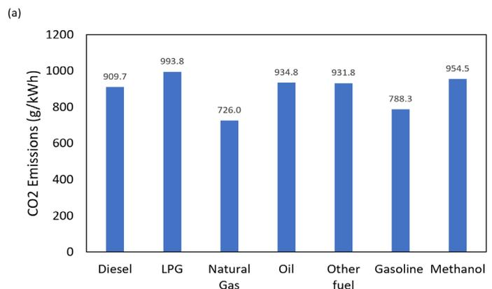
**Figure 3:** Cumulative fleet backup generator emissions comparisons of (a) CO<sub>2</sub> for different fuels.
