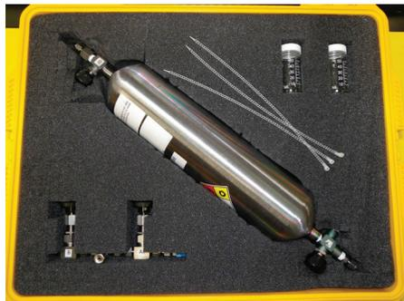
The fuel sampling kits include a 2.2-liter stainless steel cylinder [center] for collecting fuel, glass containers [top right] for collecting fuel deposit samples, and a manifold [lower left].
